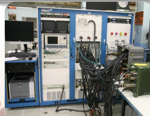
Wiring Harness Testing and Repair
