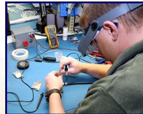
Cable and Harness Repair/Fabrication
